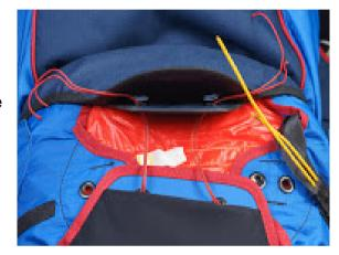
Now close the flap grommets and push the short yellow cable through the first elasticated loop and the longer yellow cable through the second elasticated loop.
