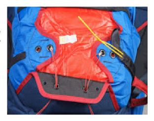
Push the packing cord through the upper flap grommet.
