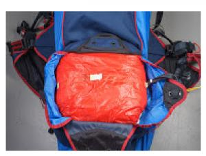
Push the packing cords through the elasticated loops and the lower flap grommet.
