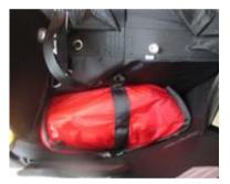
Position the split pins and release handle below the neoprene cover.
