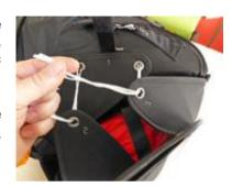
Build the parachute with the handle loop up and the lines down and insert the split pins into the respective color-marked loops (white- white, black- black).
