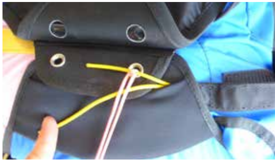
Push the yellow cable through the loop and gently pull the cord out.
