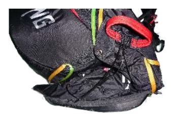
Put in the rescue-system container. The connected handle is showing to the seatboard and the container opening of the harness
