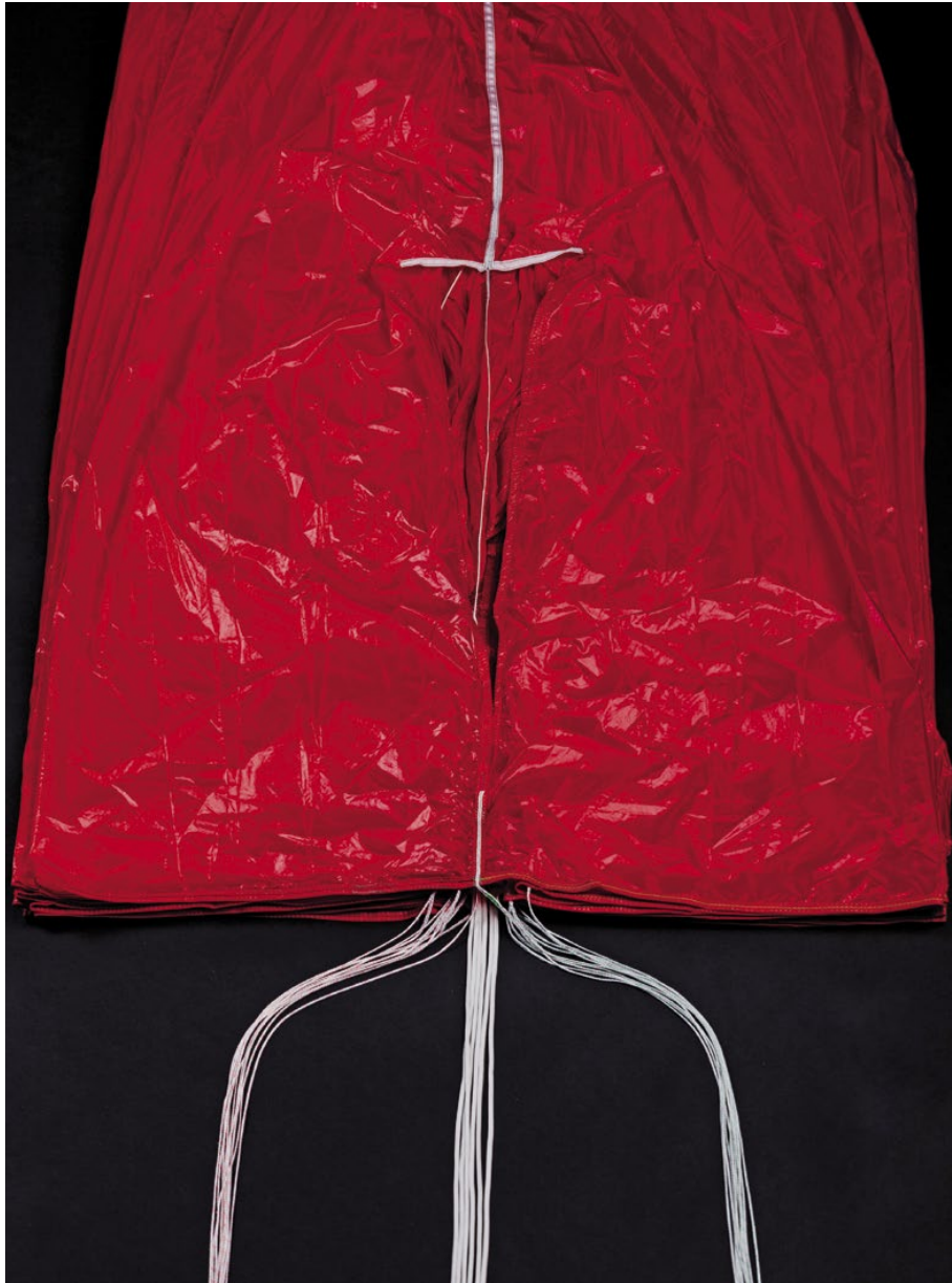
Lay out the canopy in a way that the gore is placed with the opening slot at the top.
