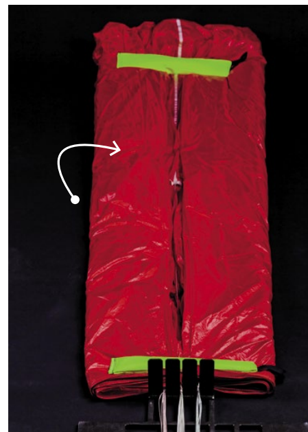
Double over the left canopy half towards the centre axis.
