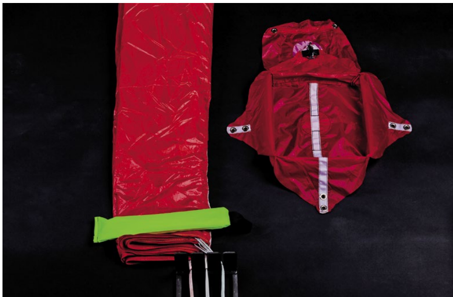
Now the canopy is folded to the correct width of the container.
