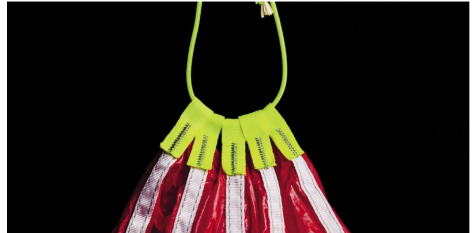
Gather the five yellow packing loops together and secure using a packing line.
