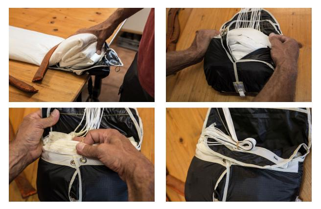
Close both sides of the inner container and the top pocket with the rubber, which you fix with one loop of all the suspension lines.
