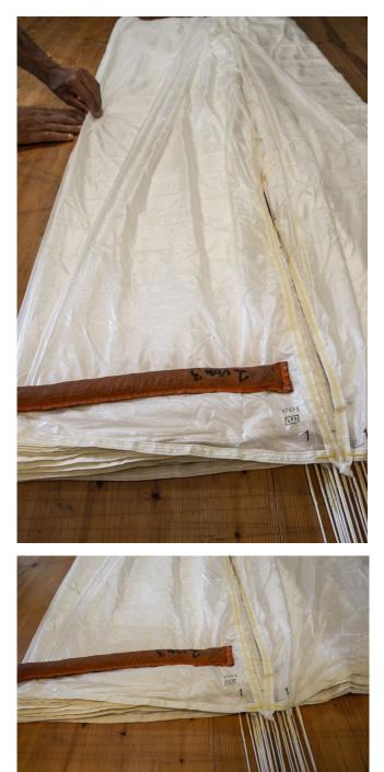
Panels with slots are laid out as cone.
