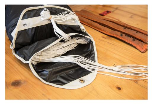
Use the last 20 cm of the suspension lines for the final closing of the inner container with the black rubber.
