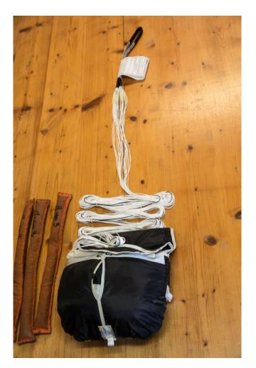
The suspension lines are sorted in three bundles, which are fixed by rubbers. These bundles are stored in the pocket of the container.
