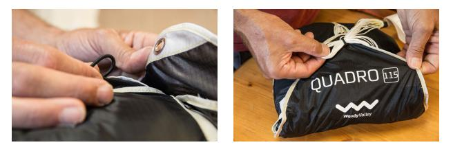
With the rest of the suspension lines you finalize the closing of the inner container by pulling the suspension lines through the black rubber loop. Don't make the closing loop to big.
