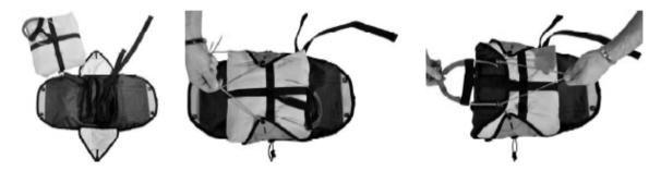
Push the plastic pins on the handle into the elastic loops and under the transparent cover. It is essential to remove the cord after this operation. The cord should be pulled out slowly in order not to damage the elastic loops by excessive friction. Lastly, the handle should be positioned under the two cover loops.
