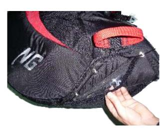
After closing the container, by putting in the pins, remove the packing cords and put the release-handle in the therefore assigned pockets
