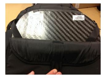
**Important:** when reinstalling the seatboard make sure it is the right way up - convex side on top when flying - and that the leg straps lie cleanly around the board.
