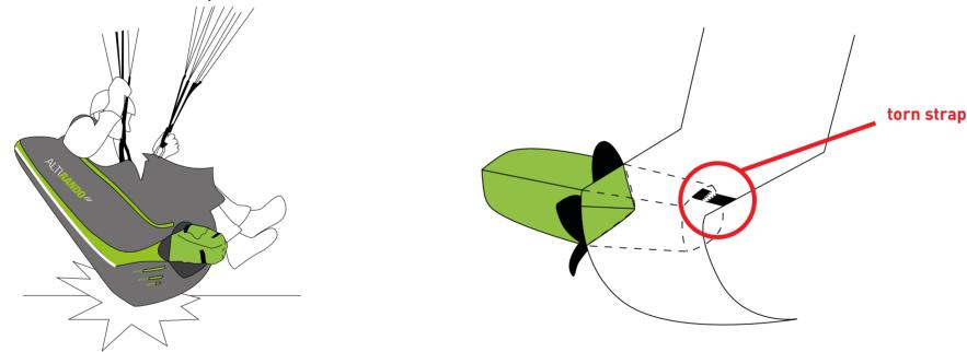
Our various tests show that the pocket damage does not take place when the reserve parachute is inside the rescue pocket (closed).
