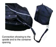
Put the bridle into the container of the hanrness. The connection to the handle must be also between the innercontainer and the harness, as shown on the picture. That means it has to be on the inner side. So you can be sure that the rescue-system can be pulled out easily.
