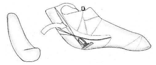
For building-in the protector you have to take care that the protector is put in the therefore assigned pockets in the protector-bag of the harness. The Velcros of protector and protector-bag have to be fixed with each other to avoid an unintentional movement of the protector.
