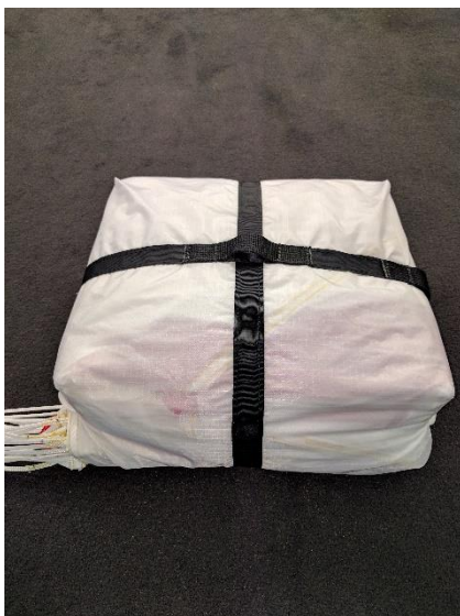
17. Flip the rescue container over the canopy. The handle attachment point should be on the opposite side of the lines.
