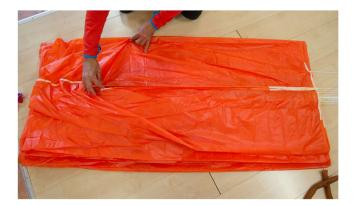
Panels with slots are laid out as cone.
