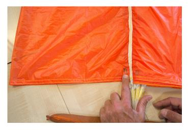
Put all the panels to the right side and fold over each panel from the right side onto left side like turning the pages in a book and pull the top of the opening outward.
