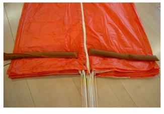
Put a packing weight for fixation on the last panel and then all the panel from the right side can be shifted to the that side.
