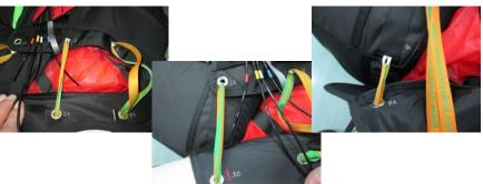
Pull the cord trough the grommets and pin all the loops with the handles closing cable from 1 to 4. For your convenience there are different color markers on each cable and each grommet.
