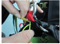
The Loop must be on the back side of the grommet. Lock with the cutaway cable and insert the cable end into the belt pocket
