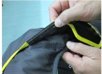
Stick the RSL line with the Velcro and after that close the pin cover flap
