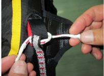
Insert the soft link line in the red attachment point (1) located at each shoulder belt ( under the magnets ), and the rescue attachment line (2).
