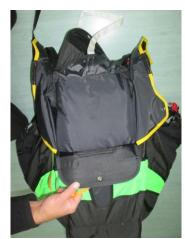
Fold the Rescue Static Line (RSL) on to the free bag.
