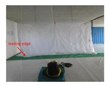
After you check all the canopy lines, lay down the harness and sort out the main risers.
