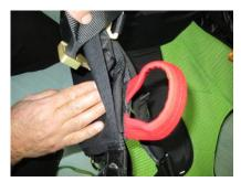
!!! CHECK IF THE CUT AWAY CABLE IS PASSING TROUGH BOT HOSING !!!
