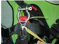
After that pass the pull up cord, from front to back, trough the loop, the small ring and the grommet.
