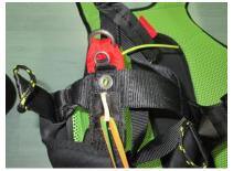
Pass the big ring trough the karabiner firs and after that the small ring trough the big one.
