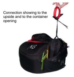
Put the bridle into the container of the hanrness. The connection to the handle must be also between the inner-container and the harness, as shown on the picture. That means it has to be on the inner side. So you can be sure that the rescue-system can be pulled out easily.
