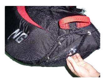
After closing the container, by putting in the pins, remove the packing cords and put the release-handle in the therefore assigned pockets
