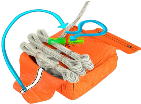
Fig 28 – Line bundles in the container, ready to close the last flap
