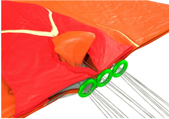
Fig 15 – Middle of the canopy bulging out
