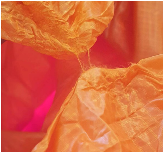
Fig 4 – Velcro damage on canopy fabric
