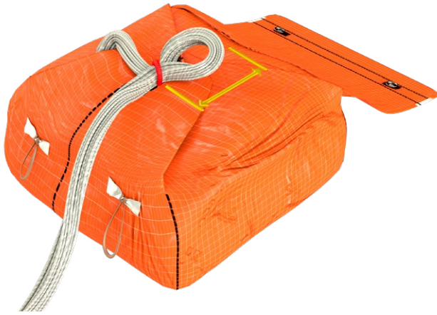
Fig 30 – Line bundles arranged, checking the diameter of the closure loop
