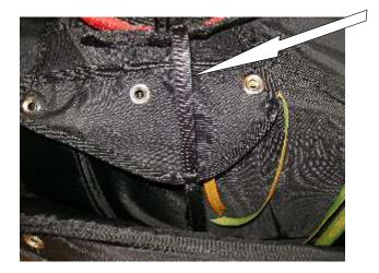
The connection to the handle runs between the two upper eyes. You have to take care that the connection of the handle is not hindered in any way and is still long enough, so that you can be sure that the pull is coming first on the closing-pins and not on the connection to the inner container!
