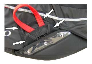
After closing the container, by putting in the pins, remove the packing cords and put the releasehandle in the therefore assigned pockets
