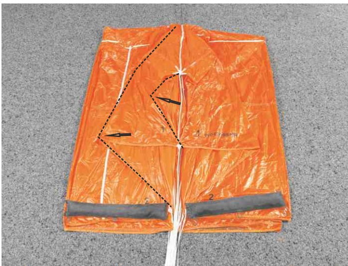
23. Arrange panel 1 (corner panel) and place a packing weight onto the periphery.
