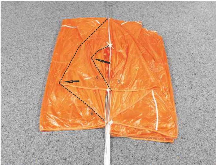
19. Arrange panel 5 (corner panel) (Evo Cross 160:panel 6)
