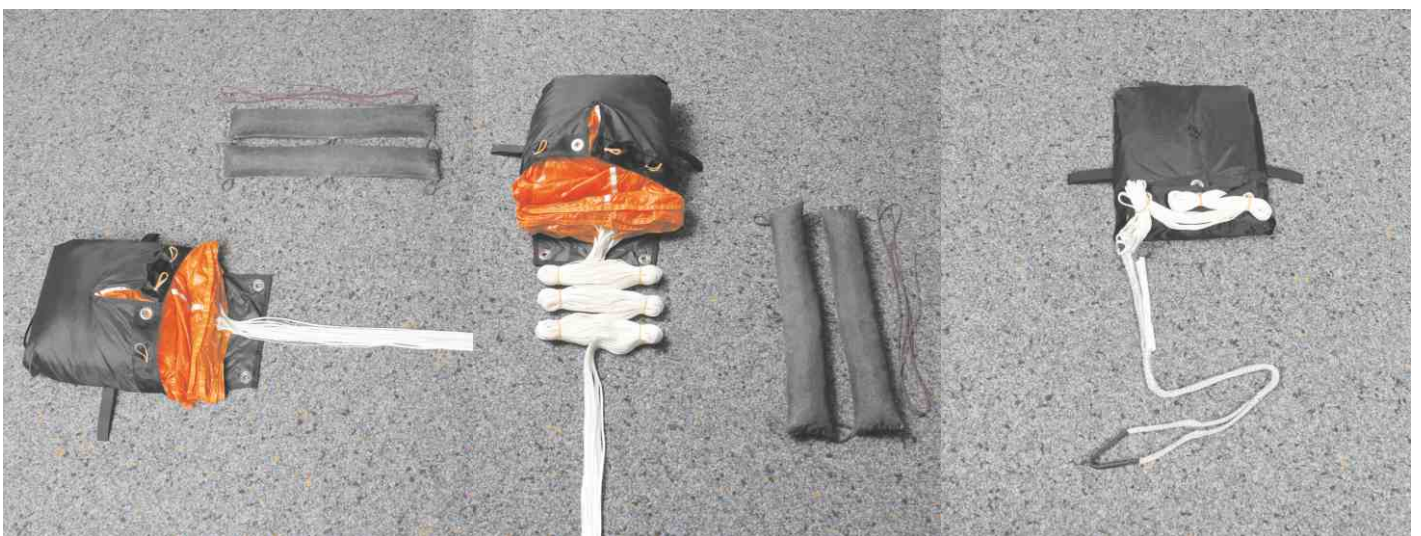
29 a. Put the S-folded canopy in the deployment bag.
