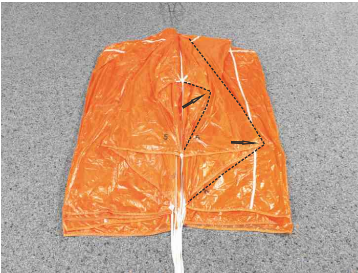
9. Arrange panel 5 (corner panel) (Evo Cross 160: panel 6)
