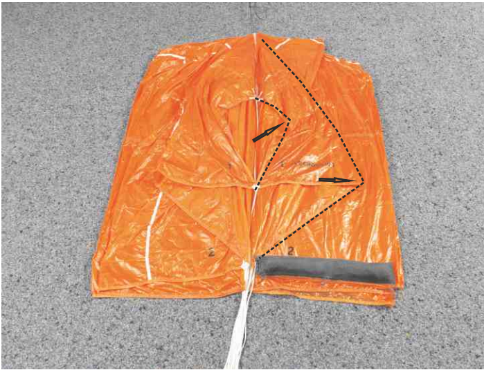
13. Arrange panel 1 (corner panel) and place a packing weight onto the periphery.
