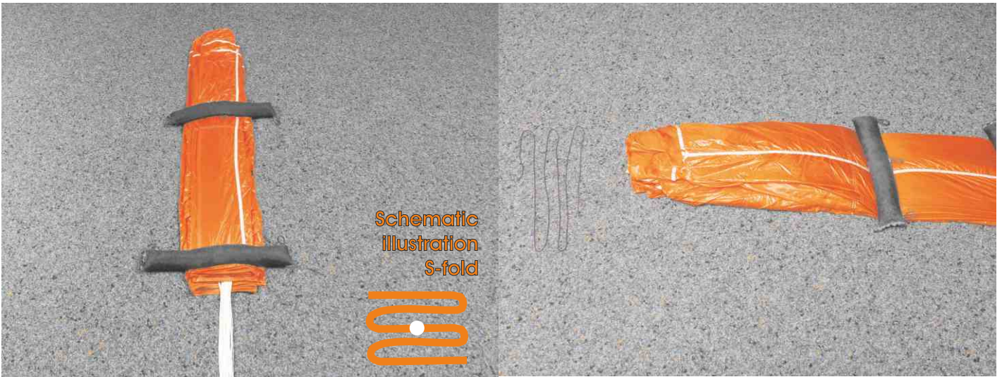
25. Fold left side S-shaped. (Step 2)
