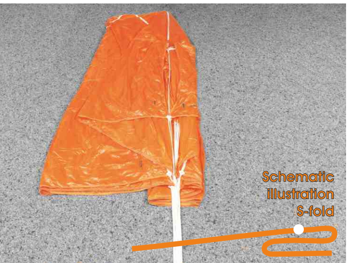
24. Fold right side S-shaped. (Step 1)
