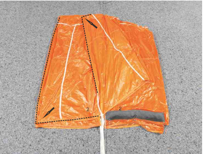
22. Arrange panel 2 and upper part of panel 1 to the side.
