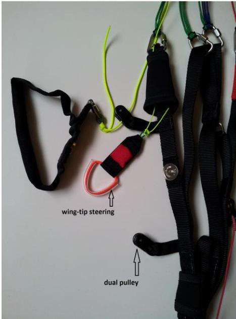
To add to the wings efficiency we have incorporated **wing tip steering** options, which allows for turning with a reduced bank angle, therefore reduced descent rate.
