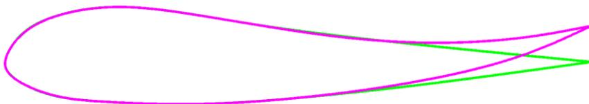
The reflex design allows the wing to transition from a paragliding configuration (green profile - for slowest flight and best lift. Best option for take-off) to one where the trailing edge is released (pink profile - Lift is compromised for speed. Reflex is installed) shifting the centre of gravity forward along the wing chord adding pressure to the leading edge. This increased pressure and diminished angle of attack along the leading edge adds speed and safety to the glider.
